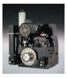
The system features improved energy efficiency, because the main servomotor and pump run only during the recovery (plasticizing) portion of the cycle. A typical hydraulic system would have the electric motor and pump running continuously, with the variable pumps destroked during idle periods.
