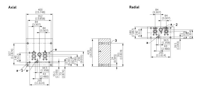
Attachment Bypass between Cylinder Chambers (Interface similar to Basic Manifold)
