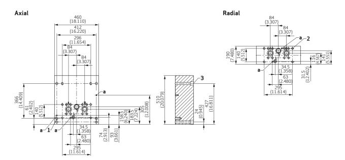
Attachment Bypass between Cylinder Chambers (Interface similar to Basic Manifold)
