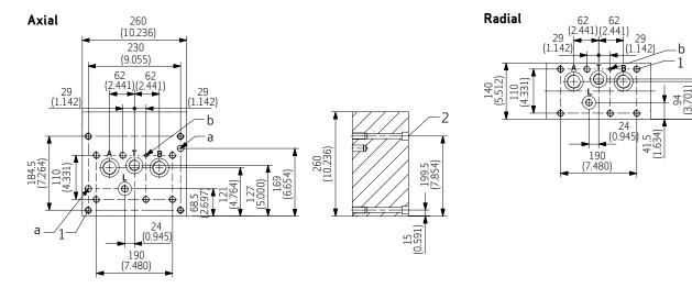
Attachment Bypass between Cylinder Chambers (Interface similar to Basic Manifold)
