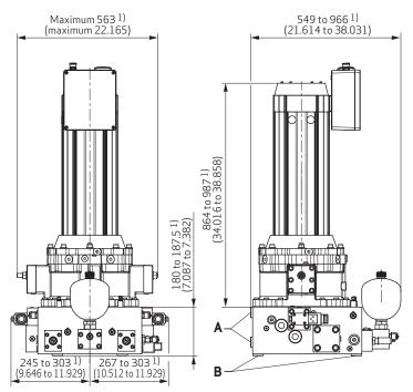
A: Distance washer for radial connection  $^{1)}\ B$ : Distance washer for axial connection  $^{1)}\$
