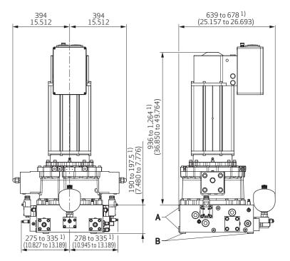
A: Distance washer for radial connection  $^{1)}\ B$ : Distance washer for axial connection  $^{1)}\$
