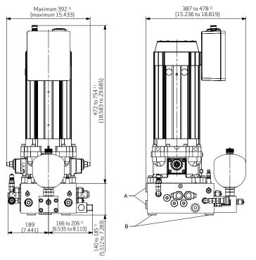
A: Distance washer for radial connection  $^{\rm 1)}$  B: Distance washer for axial connection  $^{\rm 1)}$
