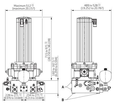
A: Distance washer for radial connection <sup>1)</sup> B: Distance washer for axial connection <sup>1)</sup>
