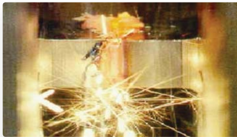
Linear-friction welding physically welds components by rubbing them together at speeds around 50 Hz and with forces as high as 800 kN. The final mass of the two titanium pieces shown is 1,500 kg.
