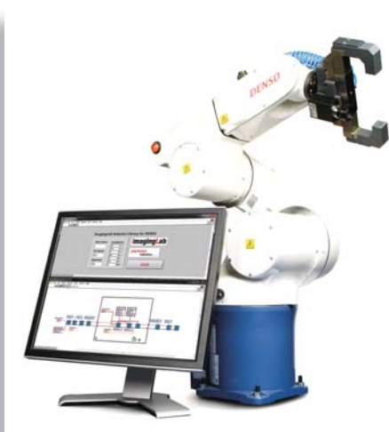
Some DENSO arms include National Instruments software and hardware to make setup easier.
