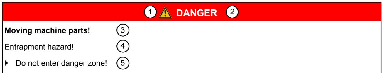
Figure 1: Structure of a warning notice
