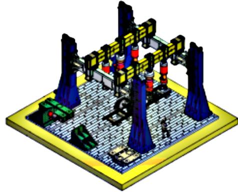
500 ton capacity 4 column portal frame for heavy duty vertical tests
