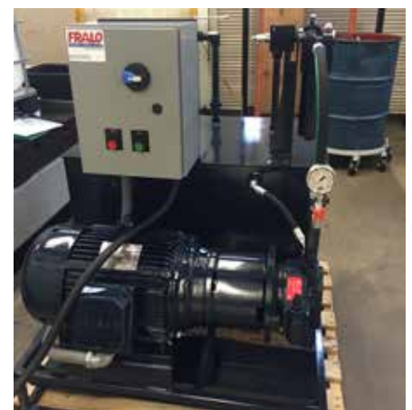
Moog-designed portable hydraulic test cart ready for shipping from the factory.
