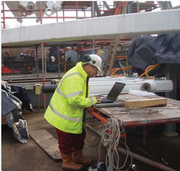
Simon Furnell from Moog tests the prototype roof in Sheffield, England. Several of the electric actuators for the end-arm assembly are visible on the table behind him.
