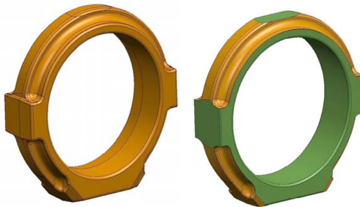
Figure 9: Sliding Stroke Ring Design: Raw Part (left) and Finish Part (right)
