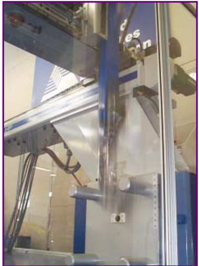
A new controller and motor configuration allows high-speed handling of injection-molded parts.
