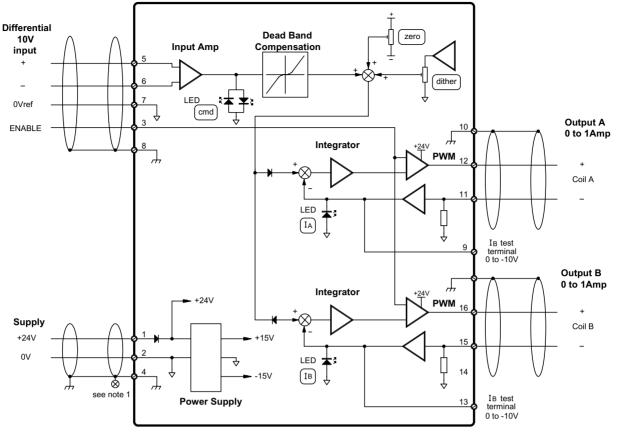
Note: 1. Connect cable screen to enclosure cable gland or chassis ground terminal on G123-814.
