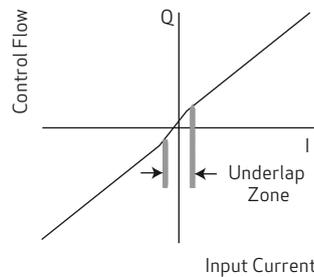
Normally used in hydraulic motor applications
