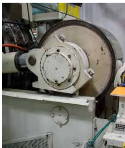
A mechanical offset on one end of the Rotocure's cylinder moved a metallic strip to the center of the roll, but does not accurately maintain the movement.
