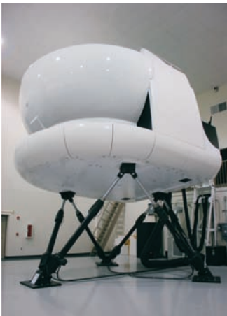
All-Electric Flight Simulator with "Stewart" 6 DOF motion platform
