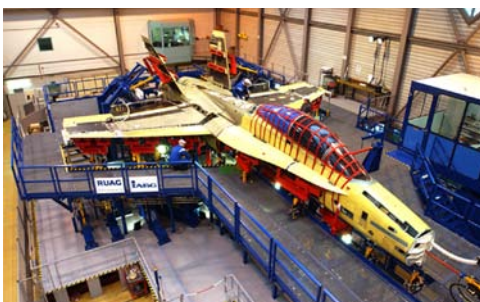
FA/18 Full scale fatigue test for RUAG, Switzerland
