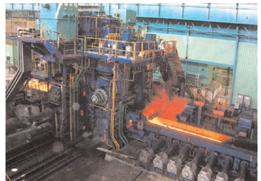
Over 100 Moog servovalves are used in this newly built 1750 Hot Strip Mill production line.
