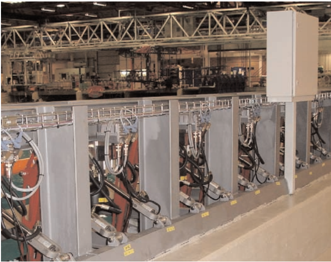
Details of multi-flap wave maker showing hydraulic cylinders and Moog Axis Control Valves
