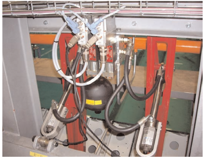
Details of multi-flap wave maker showing hydraulic cylinders and Moog Axis Control Valves
