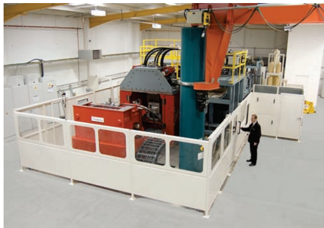
Exterior of E100 machine body in partial build, showing forge and tool assembly on the main slide
