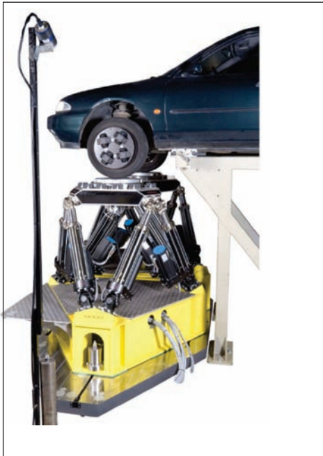
Our 6-DOF Kinematics and Compliance measurement systems have been developed in partnership with automotive manufacturers seeking highly accurate stiffness and kinematics measurements using either force or displacement control.
