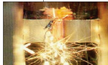
Pieces of titanium are "rubbed" together at tremendous speed (50 Hz) and with high forces (800 kN) to physically weld components to each other (mass of 1500 kg).
