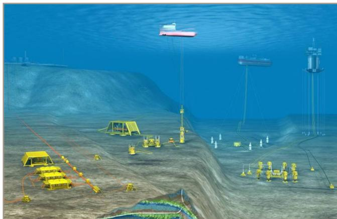
**Concept for subsea processing system**
