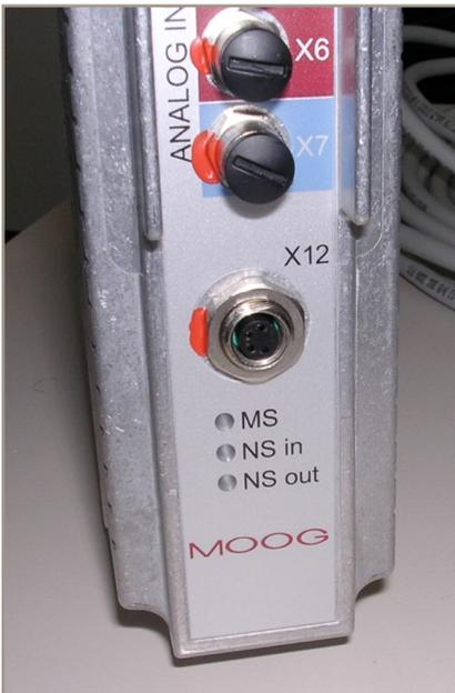
Figure 6: New analog input for sensors with resistive bridges
