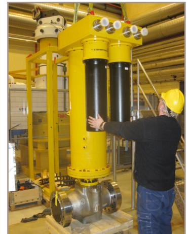
**Moog Electric Actuator mounted on Anti-Surge Valve**
