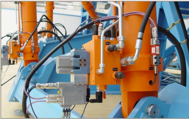
Figure 5: Cylinder with Moog D671 series valve
