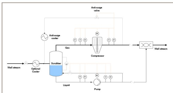
**Diagram of gas compression system showing the anti-surge valve**
