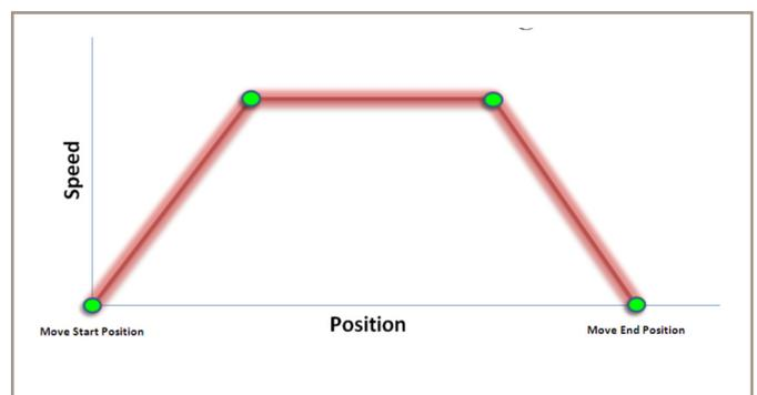
Figure 5: Electric Velocity Profiling
