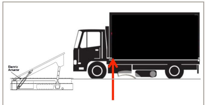
Figure 3: Penetration Measuring Location (P-Rating)
