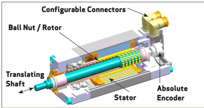
Figure 7: Cutaway of Moog Electric Actuator
