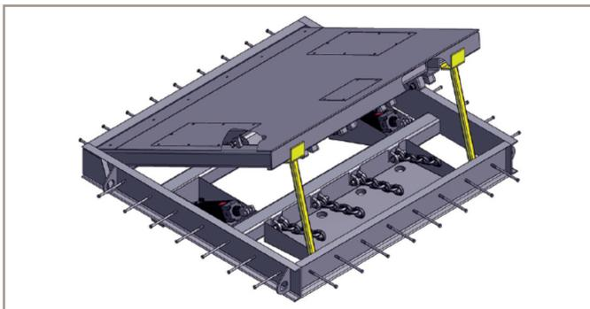
Figure 2: Wedge/Plate Barrier Construction
