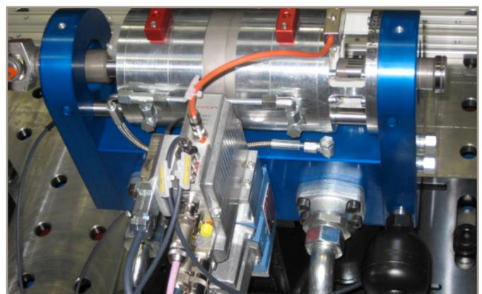
Figure 7: Moog Servo Valve with rotary drive during the test phase
