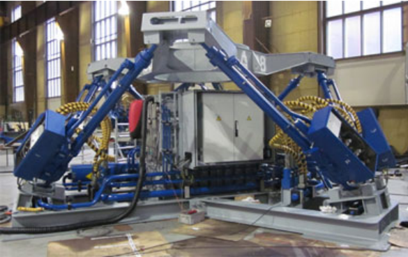
Inverted Motion Base used in Ampelmann - Source: Ampelmann
