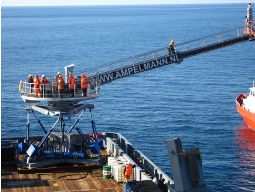
Ampelmann System Using Moog Inverted 6-Axis Motion Base - Source: Ampelmann
