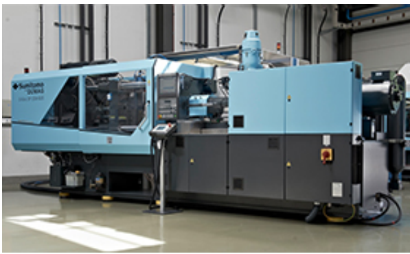
The hybrid drive high speed EI-Exis SP (shown here with 2,000 kN clamping force) has further improved dynamics compared to the preceding series. Source: Sumitomo (SHI) Demag
