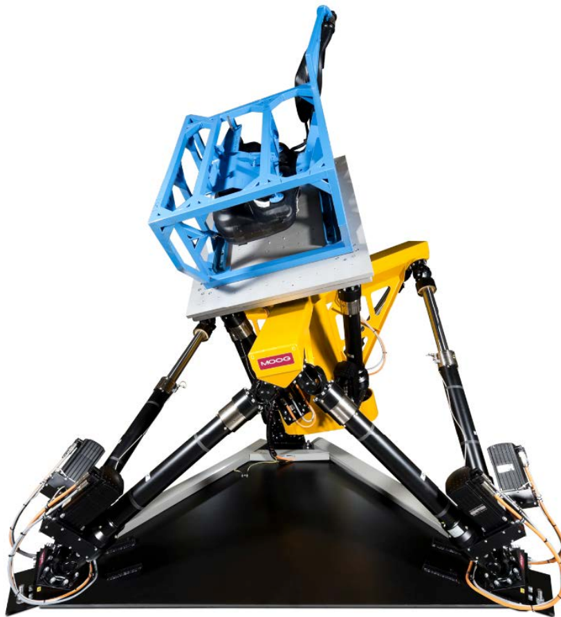
Fig. 4. 8 DOF Moog test system comprised of a 6 DOF Electric Simulation Table with an innovative extra 2 DOF tilt table.
