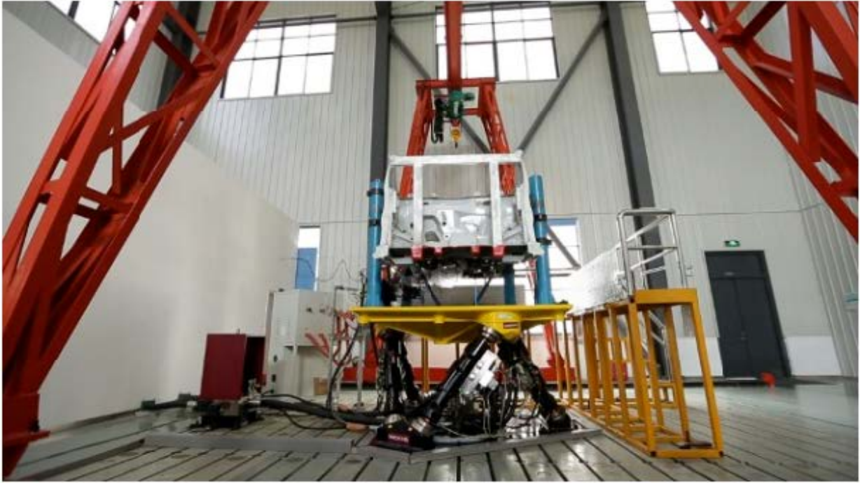
Fig. 1. Moog Hydraulic Simulation Table with a car engine mount being tested in CTI Suzhou, China
