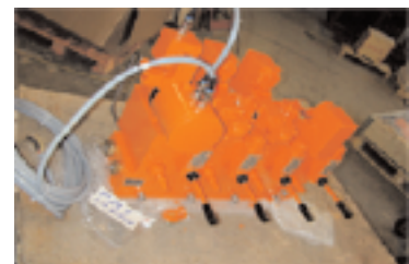
ATEX certified flame-proof Servo-Proportional valves
