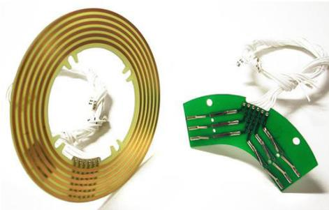
Figure 1c: Platter style assemblies
