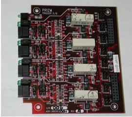
The Prizm Trigger Interface Daughtercard provides four channels of Input or Output selectable interface for use with most Acoustic Responder channels. This board is meant for use as a daughter-card on the standard PRIZM Submux1 or Submux2 motherboard. Refer to the Submux1 or Submux II manual for a description of those particular cards and the standard data daughtercards.
