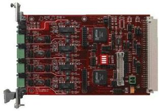
The Prizm RS-232 /422 / 485 Submultiplexer (Submux) motherboard provides four RS-232 channels that are multiplexed onto a single Prizm highspeed serial data channel. With the addition of up to three additional pluggable daughter boards, a total of 16 independent serial channels can be carried on a single Submux. The combinations of types of channels (RS-232, RS-422, and/or RS-485) will vary depending on the type and
