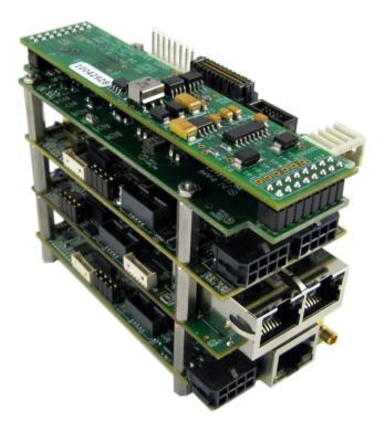
The Moog Focal 914-X Series multiplexer system provides optical data rates up to 6 Gbaud. Taking advantage of this abundant bandwidth, a series of expansion cards is available to complement the 914-HDE motherboard. These expansion options are packaged into the same credit card size form factor and stack neatly on top of the 914-HDE. Up to 8 expansion cards with various options may be stacked onto a single 914-HDE motherboard to create a feature rich yet compact modular multiplexing solution.
