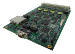
The Model 922-420 provides an advanced SIIS Level 1 gateway to a SIIS level 3 network, and is ideally suited to interface with modern control systems. It has been designed and qualified specifically for permanent subsea installation and is highly fault tolerant by using protection and redundant circuitry.
