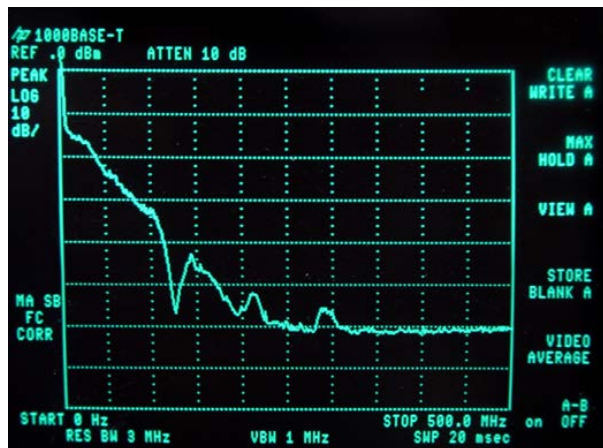
Figure 4: Frequency Spectrum of Gigabit Ethernet (1000Base-T)
