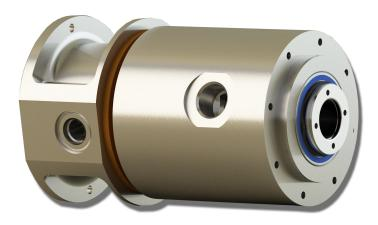
The Model 801 Fluid Rotary Union (FRU) is designed to operate with ethylene glycols (non-silicate inhibitors), propylene glycols and polyalphaolefins (PAO), providing very low leakage rates over relatively long service intervals. The Model 801 FRU can be used as a standalone unit, or can be integrated with electrical slip rings and/or fiber optic rotary joints.
