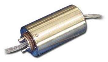
The FO300 is a prism based multichannel fiber-optic rotary joint (FORJ). It is a passive and bidirectional device which can be used as a standalone device or easily integrated into a rotary assembly, enabling transfer of high data rate optical signals across a rotating interface.
