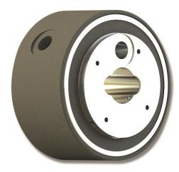
A fluid rotary union (FRU) functions as a rotary interface for fluid carrying conduit between stationary and rotating equipment. The fluid being conveyed can be liquid, gas, or vacuum. A fluid rotary union is also called a rotary union, fluid swivel, utility swivel, hydraulic swivel, hydraulic utility swivel, or rotary joint. Unlike flexible conduit, a fluid rotary union allows continuous unrestrained rotation of movable joints in machinery.
