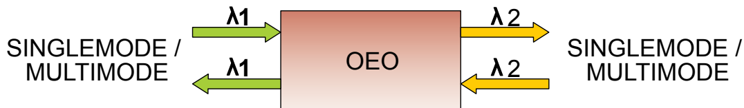
2 channel (1 bidirectional channel) Wavelength Conversion
