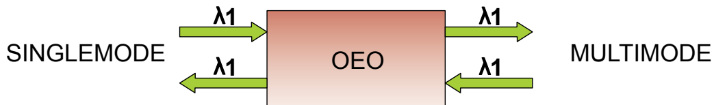
2 channel (1 bidirectional channel) Singlemode to Multimode Fiber Conversion
