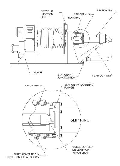
Figure 2 – Slip ring mounted outside the winch drum
