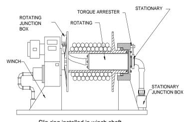
Slip ring installed in winch shaft
