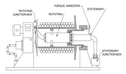
Slip ring installed in winch drum
