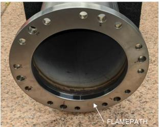
**Figure 10a** – Flamepath surfaces. It is critical that these surfaces not be damaged during removal and replacement of the COVER ASSEMBLY.
