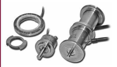
A Rotary Variable Differential Transformer (RVDT) is an electromechanical transducer that provides a variable alternating current (AC) output voltage that is linearly proportional to the angular displacement of its input shaft. When energized with a fixed AC source, the output signal is linear within a specified range over the angular displacement.
