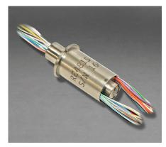
A slip ring capsule can be used in an electromechanical application to transfer low power and data over a continuous rotary interface, eliminating the need for wrapped cables. The RE4815 provides highly compact packaging to 32 conductors in a very small 1/2 inch diameter housing with an overall length of less than 1-3/8 inches.
