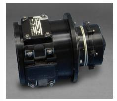
The Type 1 solar array drive assembly offers a minimum weight, minimum power solution for positioning solar array panels at the lower end of the size/power spectrum. It is based on the Moog Type 1 rotary incremental actuator. Continuous rotation of the solar array is facilitated by the integration of a slip ring assembly on the output of the actuator, and the rear accessory section of the Type 1
