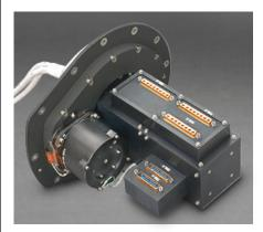
The Side-Drive Solar Array Drive Mechanism (SADM) consists of a slip ring assembly and an actuator coupled by a spur gear set, which, when driven by suitable drive electronics, will position the Solar Array toward the sun for maximum power and transfer the collected energy to the spacecraft power bus. The SADM unit is an integrated assembly of actuator, slip ring with integral position
