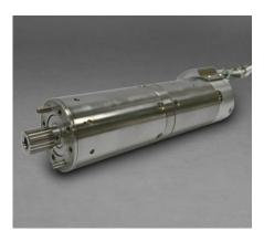
The Moog High Torque M8 rotary incremental actuator is a compact, closely integrated design made up of two key elements: a motor and a multi-stage speed reducer. The motor is a small angle permanent magnet stepper with relatively high holding torque. The multi-stage speed reducer offers a large reduction ratio (6400:1), low weight, zero backlash and high torsional stiffness. Co-axial nesting of the motor and transmission drive elements gives
