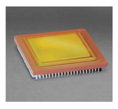
The Moog Broad Reach BRE440 CPU meets the requirements of a wide variety space and high reliability applications. The BRE440 CPU is a fully radiation hardened implementation of the PowerPC 440 processor core in a true System-On-a-Chip design, including floating point unit.
