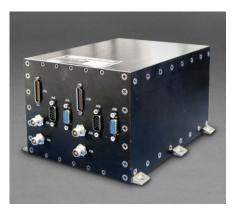
The high-reliability Gimbal Control Electronics System controls the motion of two or more motors, such as used in solar array actuators and antenna gimbals.
