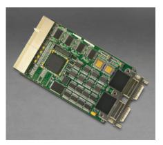
The McMOATI™ Boards (Digital & Analog McMOATI) are general purpose 3U cPCI test boards to used emulate a wide variety of payload or unique subsystem interfaces. Its intended use is for engineering and flight unit ground testing of critical space flight hardware. The board uses devices similar to those used on space flight hardware to ensure that functional and hardware compatibility are tested, even when actual subsystems are unavailable.
