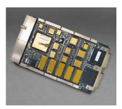
The Payload Interface Board provides a single 3U cPCI card solution to interface to spacecraft payload subsystems, with configurable real-time and high-rate interfaces and 1GByte of mass memory SDRAM.
