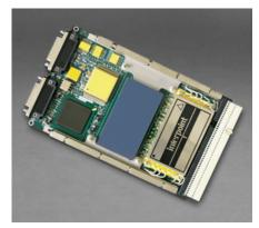
The Servo Motor Controller Electronics provides a platform for command and telemetry processing, execution of motor control commands and algorithms, execution of general purpose commands, and storage for volatile and nonvolatile data.
