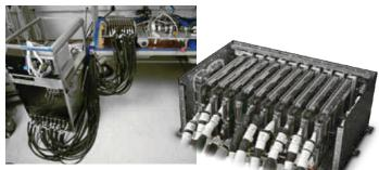
9-Joint Robotic Arm Controller System with 9 Motor Controller Boards and 1 External Communications Board
