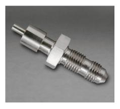
Moog cold gas thruster valves are directacting, solenoid actuated devices with a nylon poppet which is integrated in the armature/ poppet assembly. In the de-energized closed position, the armature/poppet assembly is held against the seat by a conical helical spring. The valve is opened when the electromagnetic force of the coil overcomes the spring pre-load and the armature/poppet assembly lifts from the seat allowing gas to
