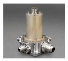
The triad isolation valve is a compact design capable of directing a single inlet of 4500 psi gas to three separate output channels. Pilot-operated, the valve has a fast response rate, making it suitable for "bang-bang" pressurization in place of mechanical pressure regulators.
