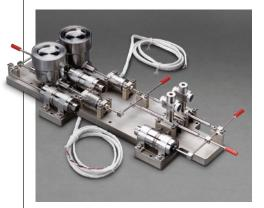
The Pressure Management Assembly (PMA) is a single fault tolerant, parallel redundant branch regulation assembly that stabilizes and controls xenon inlet pressure to a downstream, low pressure flow control device. Regulation is mechanical with no electrical input required for operation. Flow isolation is provided by latch valves, and initially with normally closed pyro valves. High and low pressure transducers are incorporated for
