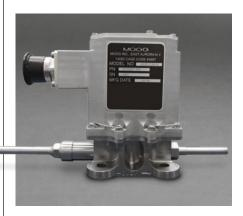
This TRL 9 high pressure latch valve is a single line, bi-stable, titanium torque motor valve, featuring integral microswitch position indication, inlet filter, and back EMF suppression diodes. This valve is human-rated, and is based on the successful heritage of Moog's torque motor valve family, spanning more than 25 years. The design features an all-welded construction utilizing wetted materials that are compatible with hydrazine.
