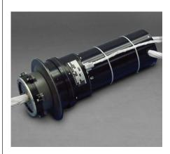
The single axis High Power Solar Array Drive Assembly (SADA) is based on the Type 5 Rotary Incremental Actuator. This standard SADA meets up to 9 kilowatts of power transfer. The design is configured with a Harmonic Drive gear set driven by a Moog discrete permanent magnet stepper motor, potentiometer for position sensing and a high power slip ring assembly for power transfer.
