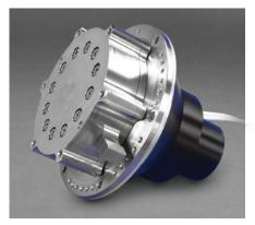
The Moog Micro3 rotary incremental actuator is a compact, closely integrated design made up of two key elements: a rotary actuator and a standard Type 3 speed reducer and output flange. The motor is a small angle permanent magnet stepper with relatively high holding torque. The multi-stage speed reducer offers a large reduction ratio, low weight, low power consumption, zero backlash and high torsional
