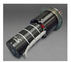
The single axis Type 3/5 Solar Array Drive Assembly (SADA) is based on the Type 3 Rotary Incremental Actuator with a Type 5 sized Harmonic Drive gear transmission and output duplex pair. This standard SADA has varied over many applications to meet mission requirements. Generally, the items that tend to vary are interface parameters and power transfer requirements. All of the represented
