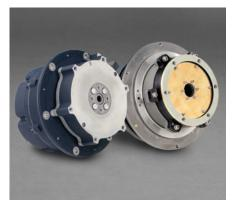
Along with the standard Type 3 and Type 5, the Moog Type3-EF and Type 5-EF Rotary Incremental Actuators are new additions to the rotary incremental actuator lines. The design is based on a recently developed ultra fine step angle permanent magnet stepper motors which in combination with the standard harmonic drive gear reducers produces extra fine output step resolution. The new line of
